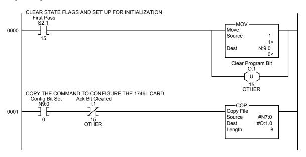
When the configuration command is complete, the program will copy the LDT configuration command for LDT 1 into the output image table with the programming bit set. This command will configure LDT 1 for the speed of wire, count direction, recirculations, and LDT length. The speed of wire for LDT 1 is 9.300µs/inch. The counts are defined as increasing from the LDT head. There is only 1 recirculation and the LDT length is 12.0 inches. This continues until the command has been acknowledged.
