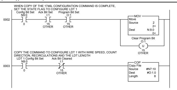
When the LDT configuration data has been acknowledged for LDT 1, the program will copy the configuration data for LDT 2 into the output image table. The speed of wire is defined as 9.272µs/inch. The counts will be increasing from the LDT head. There is one recirculation in the LDT and the LDT length is 24.0 inches. This will continue until the command is acknowledged by the 1746L LDT Interface Module.
